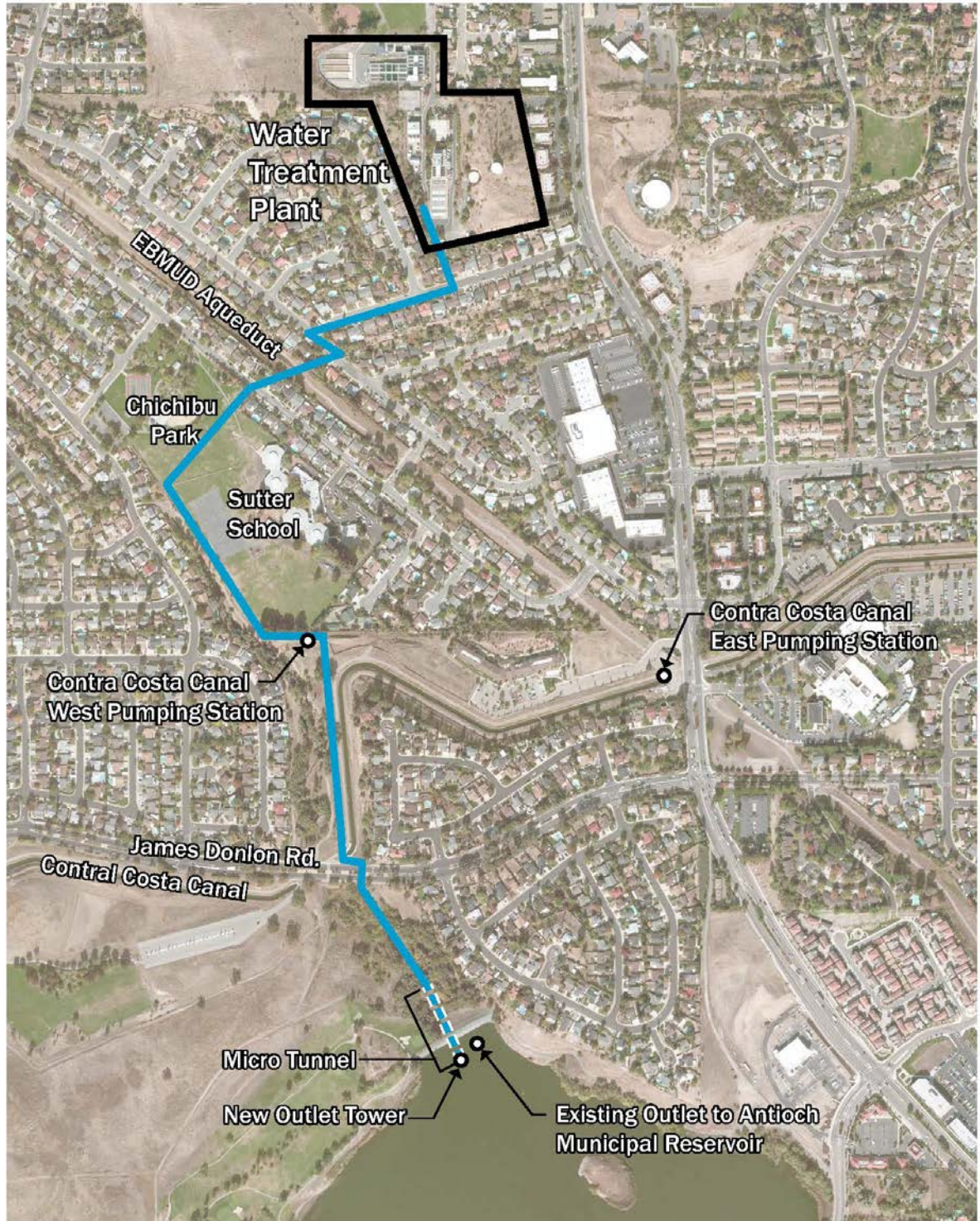
Figure 5-2. Preliminary Route for New Raw Water Pipeline from Antioch Municipal Reservoir to Water Treatment Plant
